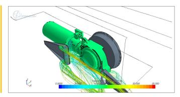
volume of the bogey cavity is very limited as the bogey can move relative to the tram.
